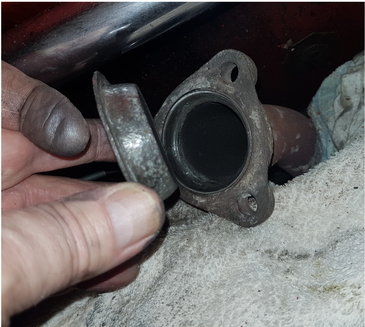
Exhaust protruded above flange
